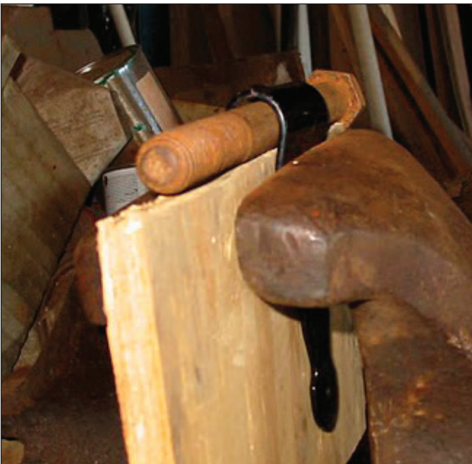
Donn then used a vice to fit the clips to the thickness of the tug. The bolt at the top ensured the sleeve and harness bolt would later fit easily. He then put in the sleeve as he prepared to hammer in the rivets to hold the clip in place.
