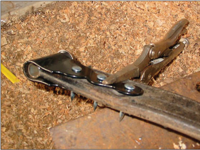
The mild steel rivets are driven through the clips and tug, clipped off and hammered down.
