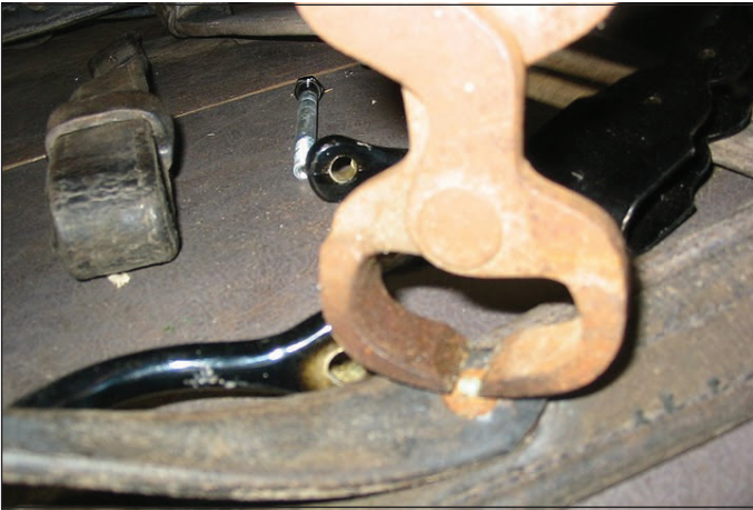
The rivets are cut off with a set of nippers and the holding strap is pried off the tug with a screwdriver.
