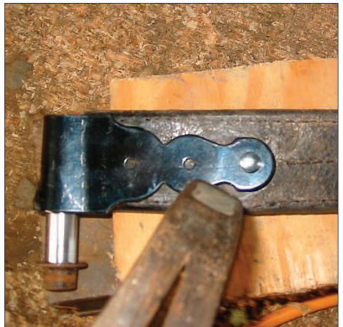
Donn then used a vice to fit the clips to the thickness of the tug. The bolt at the top ensured the sleeve and harness bolt would later fit easily. He then put in the sleeve as he prepared to hammer in the rivets to hold the clip in place.
