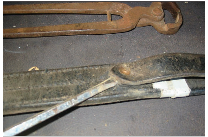
The rivets are cut off with a set of nippers and the holding strap is pried off the tug with a screwdriver.
