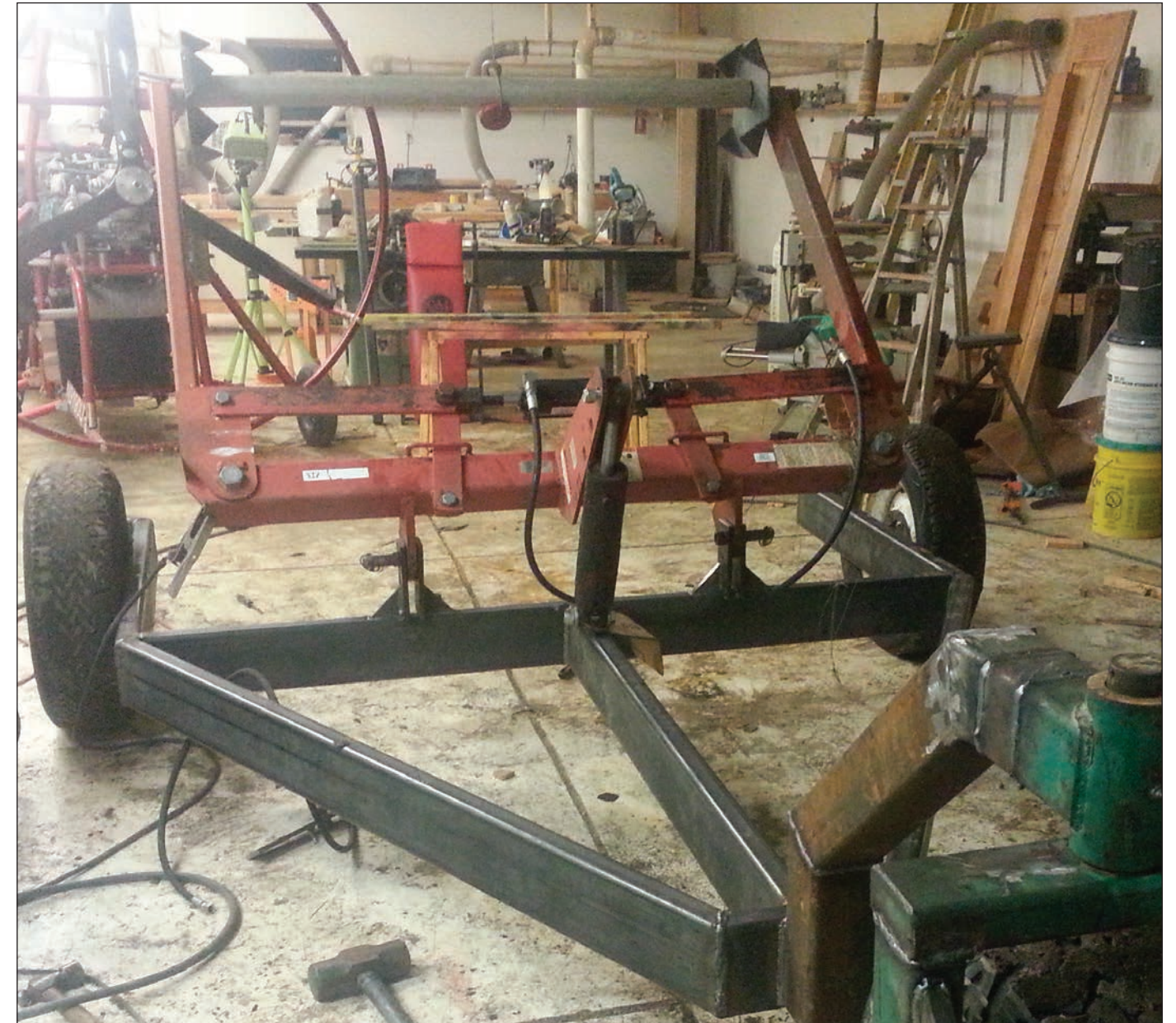
Wes located a Worksaver three-point hitch unroller and Kari fastened it to the wishbone frame.
