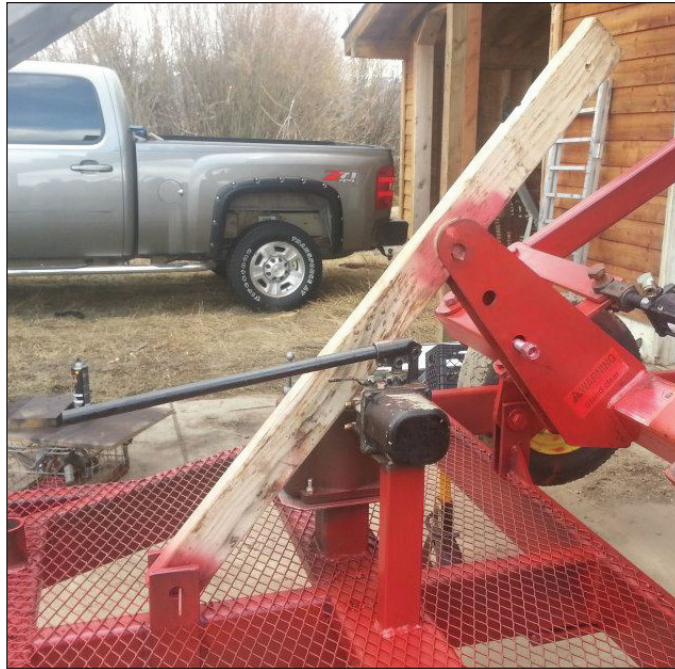
Kari used a 2x4 to take the place of the hydraulic ram that was on order during the later stages of construction. The smaller hydraulic pump shown here was salvaged from a cab-over truck and is used to run the "squeeze".
