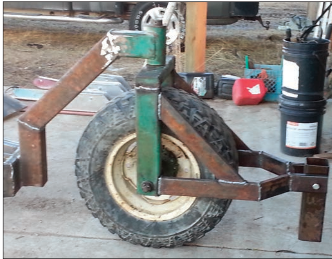
A crazy wheel from a Lockwood potato planter provided the unroller's front wheel.
