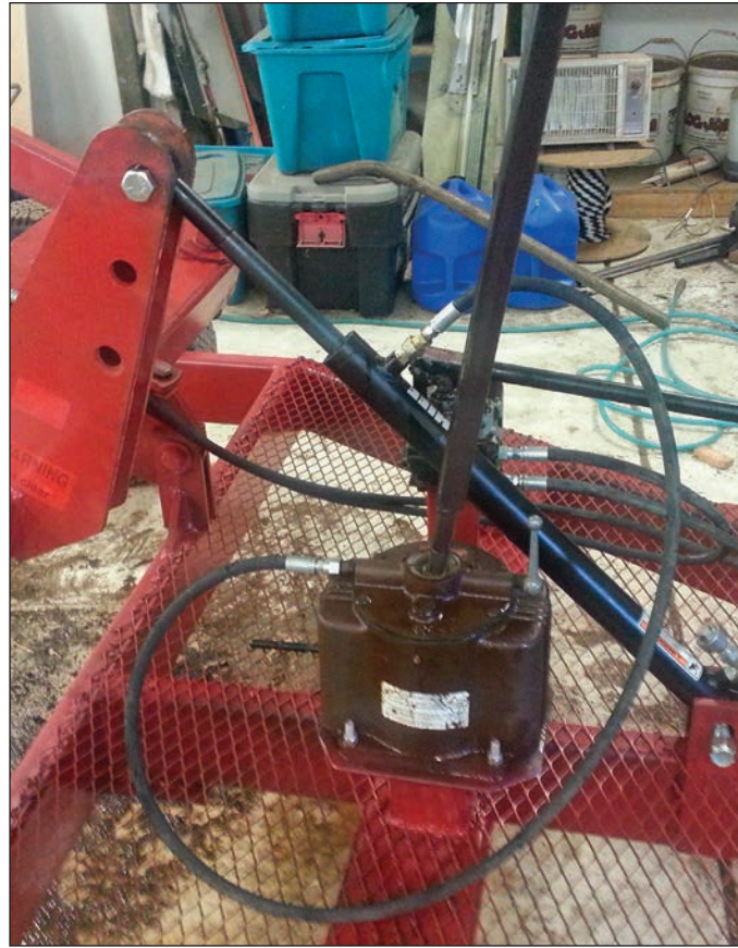
This photo shows the larger pump that operates the now-installed hydraulic ram to raise and lower the round bale.
